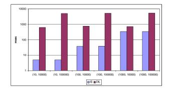
Figure 9: Finding all query answers (evaluating the Indexed Stack algorithm and DIL): queries contain two keywords; frequencies shown on X-axis
