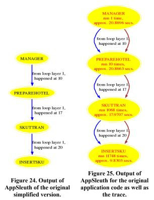
The graph of Figure 25 shows that the delinquent design pattern starting at *preparehotel* is in fact a superdelinquent, because the total elapsed time is large and the number of subroutine calls grows as one descends the tree from 10 calls to 1068 calls to 11748. (We applied both the Oracle SQL Tuning Advisor and Quest SQL Optimizer, but neither recommended any changes.)
