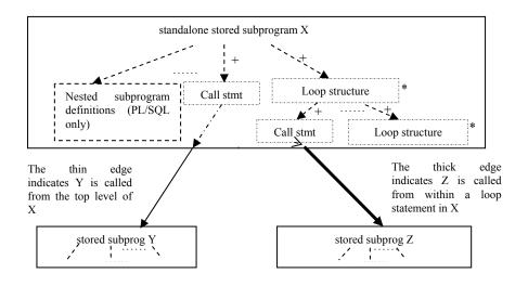
Figure 11. AppSleuth's anatomy of subprograms and two kinds of edges between caller and callee in its output. Inside subprogram X, dash lined arrows with sign '+' means multiple call statements or loop structures may exist; sign '\*' near loop structures means these structures can be nested to arbitrary depth. We omit other kinds of information using ellipsis.
