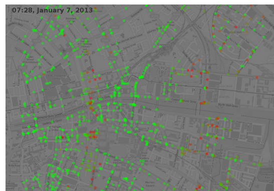
Figure 9: Traffic Flow estimates obtained by Gaussian Process Regression. Green dots correspond to low traffic whereas red dots indicate congested locations.
