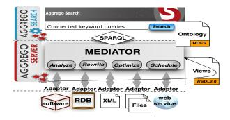
Figure 6: Architecture of AGGREGO toolbox
