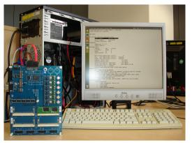
Figure 5: OpenSSD connected to the test-bed.
