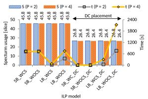
Figure 2: Spectrum usage and time as a function of ILP models for 2 and 4 candidate paths for 20 demands.
