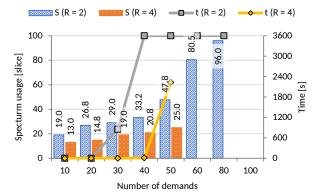
Figure 9: Spectrum usage and time as a function of number of demands for SB\_WOCS\_DC for 2 and 4 DCs
