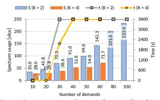
Figure 5: Spectrum usage and time as a function of number of demands for SB\_WOCS for 2 and 4 fibers per SMFB.
