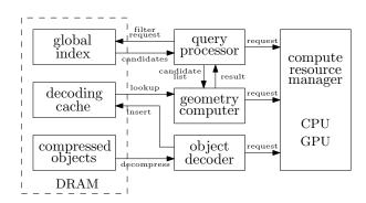
Figure 8: Overview of the architecture of 3DPro
