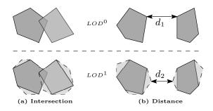
Figure 6: Properties of querying multiple LODs
