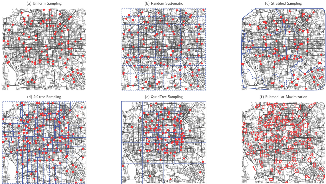
Figure 4: Sampling communication sensor location using road network of Beijing. (a) uniform sampling. (b) systematic sampling. (c) stratified sampling. (d) kd -tree sampling. (e) QuadTree sampling. (f) Regions (red) selected by submodular maximization given a set of queries (queries are not shown).
